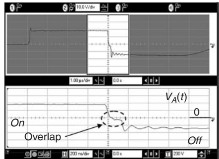
FIGURE 8-10e, f When zooming in on the secondary side anode, actually the primary voltage scaled down by N , the overlap area emerges clearly.
